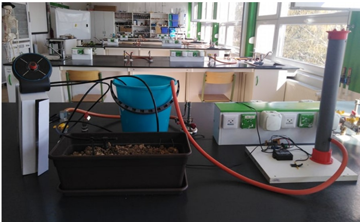
3 th picture: Model of automated water collector system
